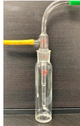
Figure 6: AGI-30 Impinger, Ace Glass Inc. Vineland NJ.
