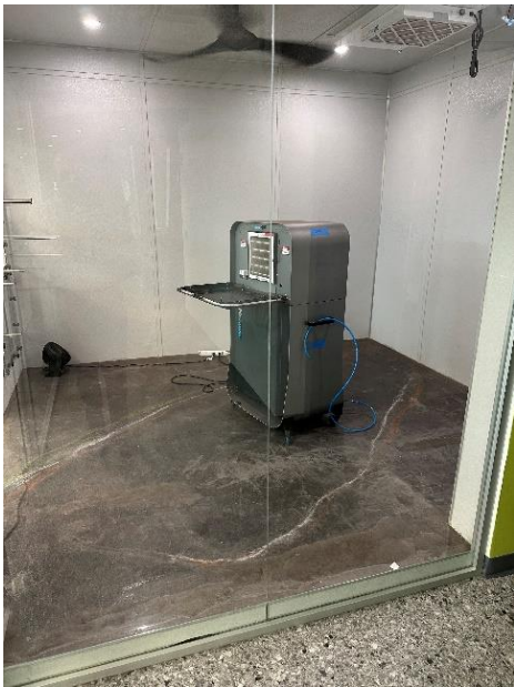
Figure 4: The CerroZone Mobile device in the 30 m 3 bioaerosol testing chamber at ARE Labs adheres to AHAM AC-5 standards and ASHRAE 241 criteria. The chamber is equipped with HEPA filtered air in/out, multiple bio aerosol sampling ports, decontamination, and pressure balance.
