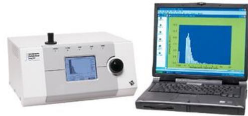
Figure 7. TSI Aerodynamic Particle Sizer (APS) model 3321 used to measure total particle concentration and particle size distribution of the challenge bioaerosol. It has a range of 0.54-20.0 µm aerodynamic diameter, with 1 particle/L detection limits.
