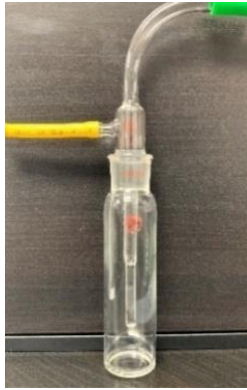
Figure 5: AGI-30 Impinger, Ace Glass Inc. Vineland NJ.
