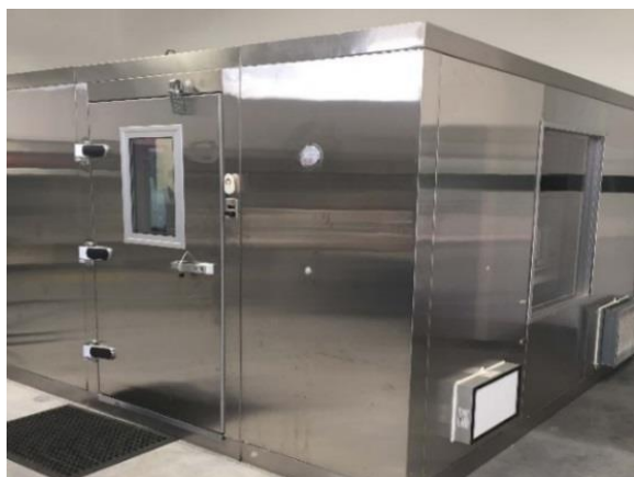
Figure 4. Testing Chamber External View The environmental test chamber used to replicate a small room environment.
