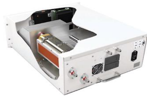
Figure 5. Thermo Fisher MAX-IR FTIR Spectrometer was used to measure gas concentrations of all chemical compounds in the air. The front of the gas analyzer is shown on the left, and the rear and internal picture is shown on the right.
