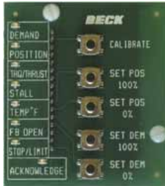
DCM-2 Pushbutton Panel
