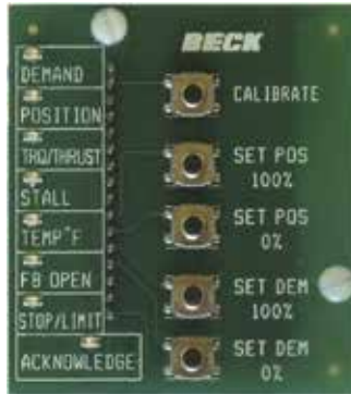
DCM-2 Local Pushbutton Panel
