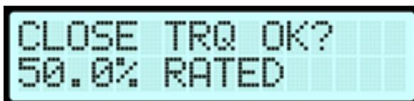
If the current value is acceptable, toggle the handswitch to YES. To change the value, toggle the handswitch to NO. Releasing the handswitch will increment the value. Holding the switch in place will continuously increment the value; slowly at first, but more quickly as the switch is held in the NO position. The values can only be increased, so if the desired value is passed, continue holding until the desired value is displayed once again.
