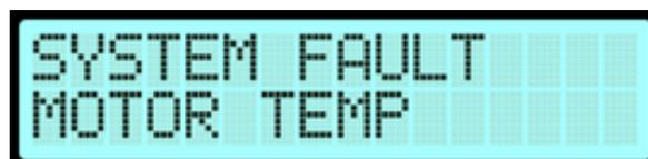
**NOTE:** Once a fault occurs in the system, the system is prevented from operating without operator intervention. Faults may be cleared by the user if the fault is no longer occurring in the actuator. To clear the fault, set the handswitch to STOP, then hold the OPEN/CLOSE handswitch in the OPEN or CLOSE position for at least 3 seconds. The display should revert back to the POSITION status indication if the fault has successfully cleared.
