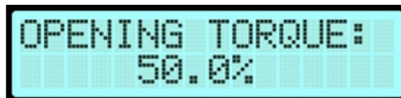
This message displays the actuator torque as a percentage of the open torque limit. Once the torque reaches or exceeds 100% of the open torque limit, the OPEN status message will appear and the actuator will stop movement.
