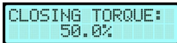
This message displays the actuator torque as a percentage of the close torque limit. Once the torque reaches or exceeds 100% of the close torque limit, the CLOSED status message will appear and the actuator will stop movement.
